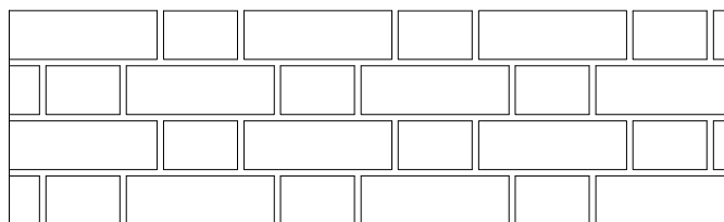
FLEMISH BOND Header / Stretcher pattern
