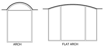
Note: The aluminium frame may be used as temporary formwork during construction. Ensure aluminium is protected and a 2mm gap is allowed for between brick and aluminium.
