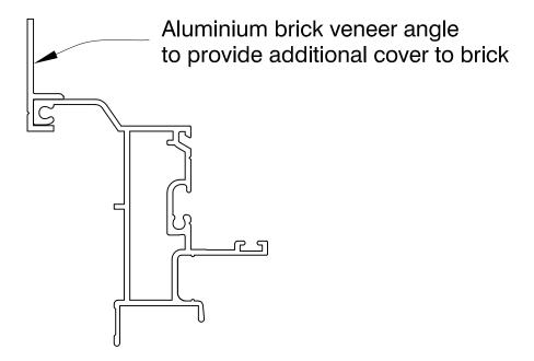
'Altherm' Aluminium Awning window frame and brick veneer angle No. 0328
