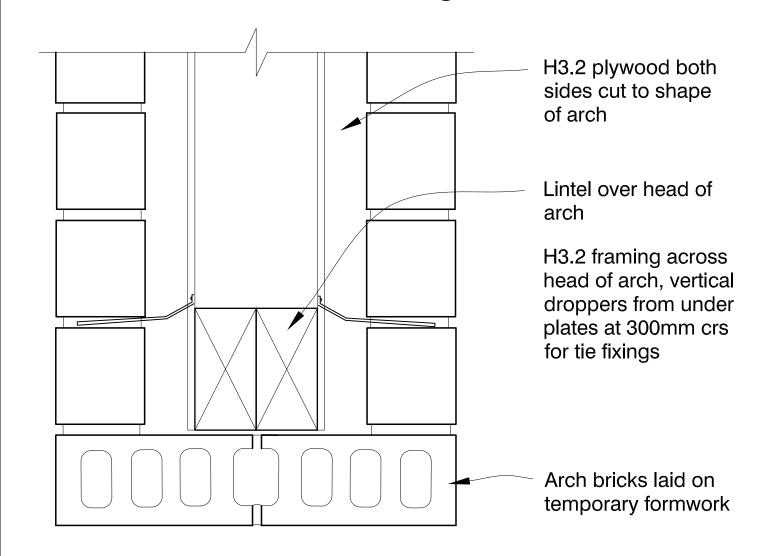
Note: Use timber wedges between arch formwork and bricks for easy removal of formwork.
