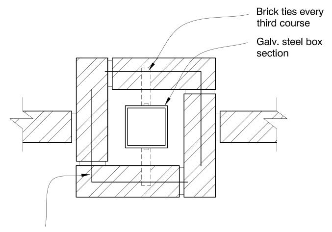
MASONS Bricklock CNR every sixth course each side, alternate the MASONS Bricklock CNR over the height of the post
