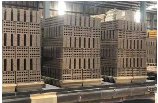
Figure 2.3 Drying of extruded bricks prior to firing
